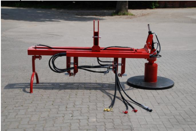
**The hydraulically driven fleece disc with control** requires a pressure port with a maximum **50l/min** and a pressure-free return flow of min. DN12
