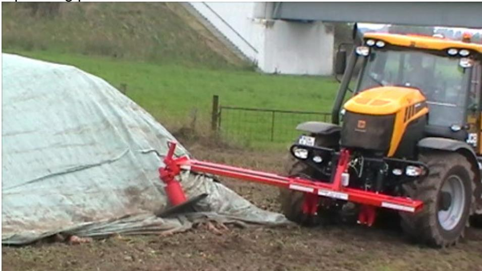
The device is swung about 5 cm from the vertical to the front in the operating position. The plate is only to be extended to the extent necessary to prevent the beets from getting damaged by the tyres
